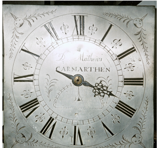
Fig. 6. A single-sheet square dial, signed by David Mathews of Carmarthen (and Talley), on a simple 30-hour country clock; the engraver is not known, author's photograph.
