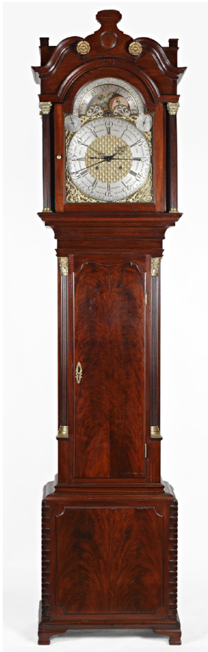
Figs 2 and 3. These images of the clock and dial show small subsidiary dials to the left and right under the fixed arch: neither of these is driven by the clock, they are set manually, both are important when forecasting the level of high water at the next tide. The chapter ring shows coastal locations between the hours; when the hour hand points to each name it will be approximately noon or midnight there. Several other clocks incorporate this feature for calculating the time at various locations throughout the world. The place names, in this case, all west of Liverpool, cross the Atlantic and are dotted around the Americas and across the Pacific.
