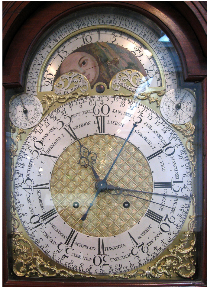
Figs 2 and 3. These images of the clock and dial show small subsidiary dials to the left and right under the fixed arch: neither of these is driven by the clock, they are set manually, both are important when forecasting the level of high water at the next tide. The chapter ring shows coastal locations between the hours; when the hour hand points to each name it will be approximately noon or midnight there. Several other clocks incorporate this feature for calculating the time at various locations throughout the world. The place names, in this case, all west of Liverpool, cross the Atlantic and are dotted around the Americas and across the Pacific.
