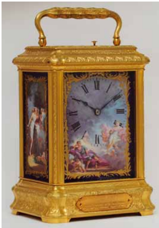
Fig. 1. Drocourt Neave Clock. c. 1885-92. 25 (handle up) x 14 cm. Fully engraved giant gorge case, porcelain dial and panels. Oversize platform escapement. Eight-day duration. Strike and repeat on a gong. Private collection.
