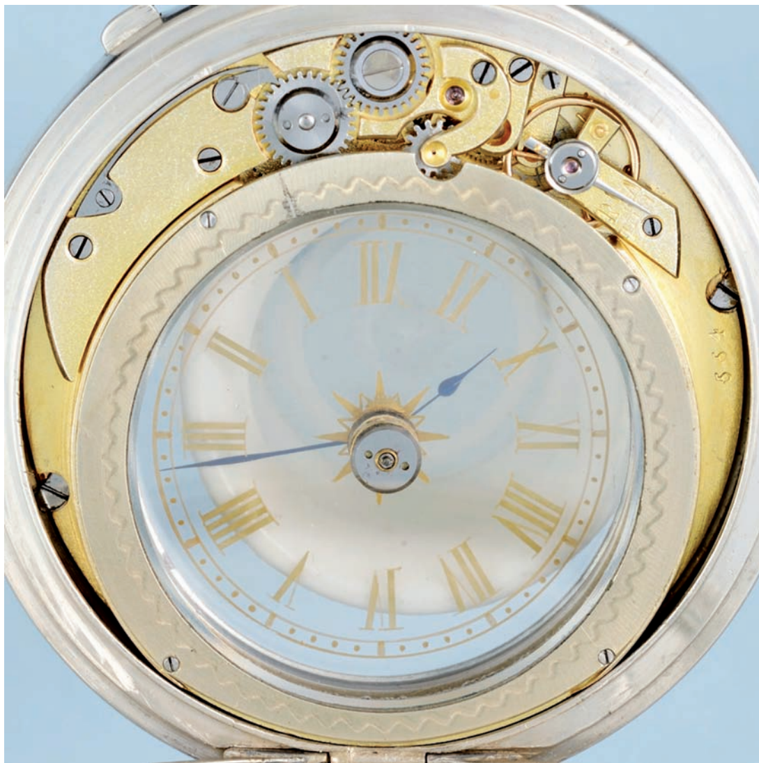
Fig. 11. SN 554 (private collection). A novel design in watchmaking back in the day, the unusual calibre incorporates a glass disk as a working part. Courtesy: Pieces of Time.
