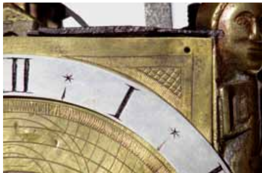
Fig. 20. Simple wobblework decoration in the corners of the dial and inside the chapter ring.
