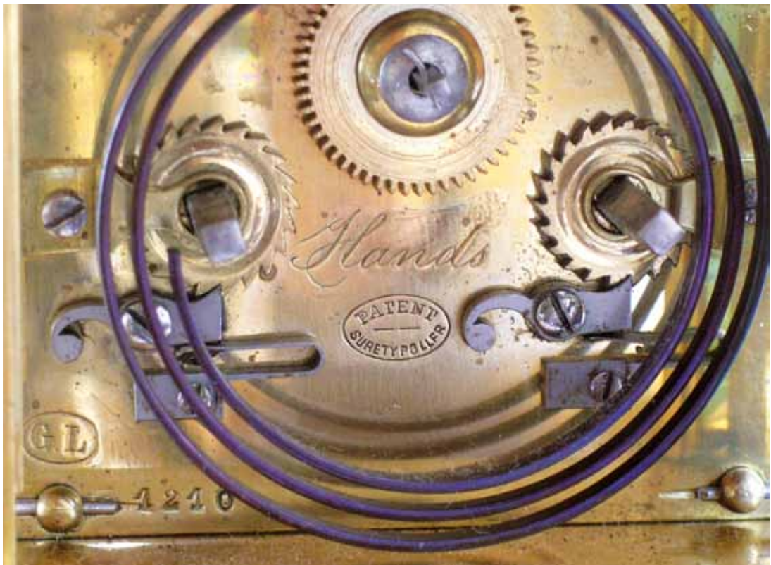
Fig. 2. Close-up of backplate of the clock in Figs 1a and 1b showing the three items of interest – PATENT SURETY ROLLER, the initials G.L, and the movement number, which on this clock is 1210.
