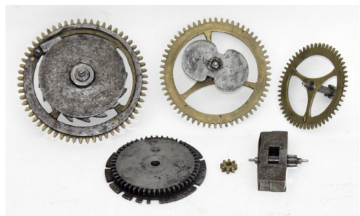
The brass wheels of the striking train, the iron countwheel and its gear wheel, and the very thick iron fly. The 'double heart' on the arbor of the second wheel provides overlift for the nag's head strike.
