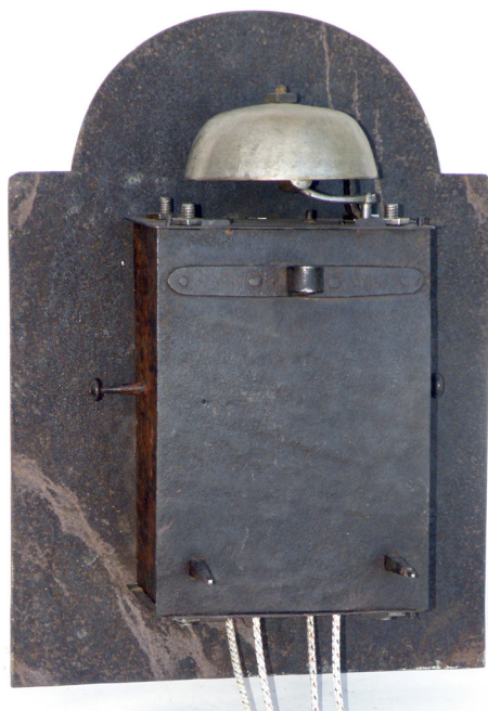
Rear of dial and case showing the hanging hoop, and spikes, with the bell fitted to the top of the case.
