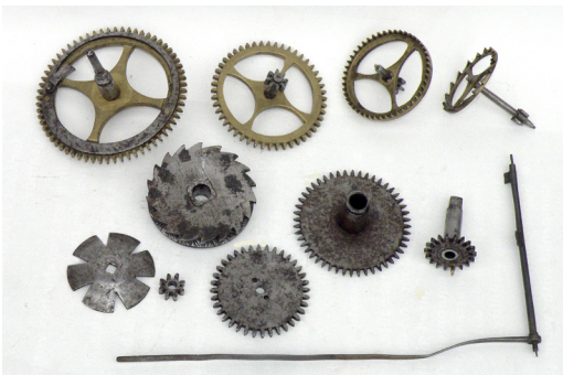
The brass wheels of the going train, the iron motion-work and verge pallets.
