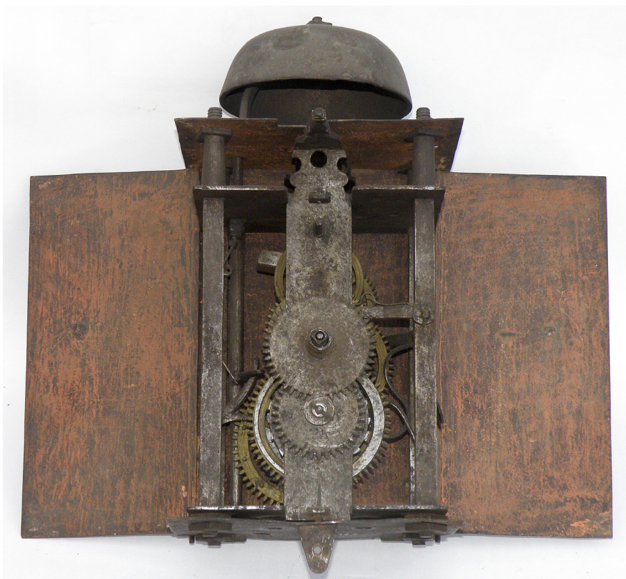
Rear of dial and case showing the hanging hoop, and spikes, with the bell fitted to the top of the case.
