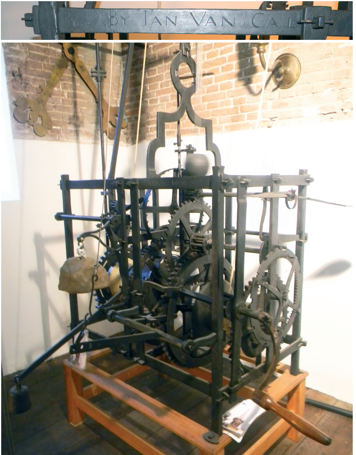
Figs 6a-b. The turret clock by Jan van Call, 1665, made for the church of St Lambert's in Buren, recently repositioned in and reinstalled in the bell tower of the church of St. Peter's in Amsterdam-Sloterdijk, and a detail of the inscription on the upper frame strip. Photographs by the author.
