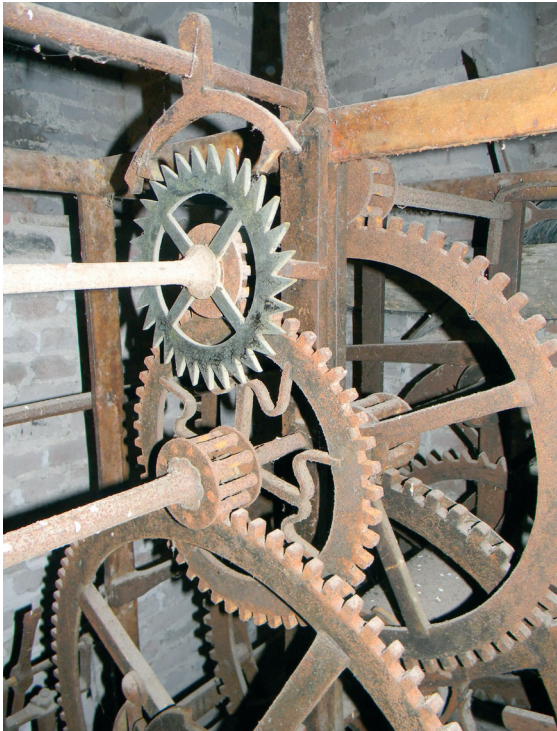
Fig 4c, Detail of the movement of the Ophemert turret clock showing the anchor escapement. Photograph by the author.
